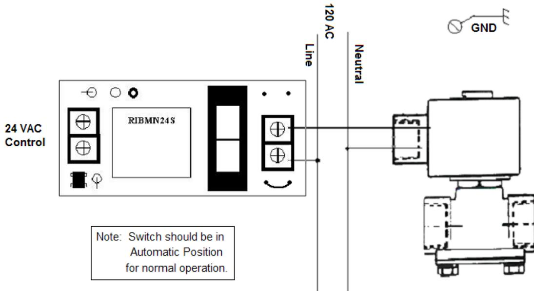
**Note:** Relay may be provided without NO or NC buss wiring removed. Installer should verify whether application requires a normally open or closed solenoid, and cut the appropriate buss wire on the relay pcb.
